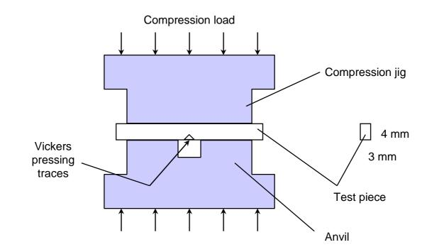
The compression load is increased until a 'popping' sound is detected, and then the test piece is immediately removed from the load.
